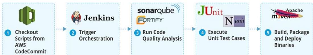
Figure 8-13. AWS CI pipeline example
